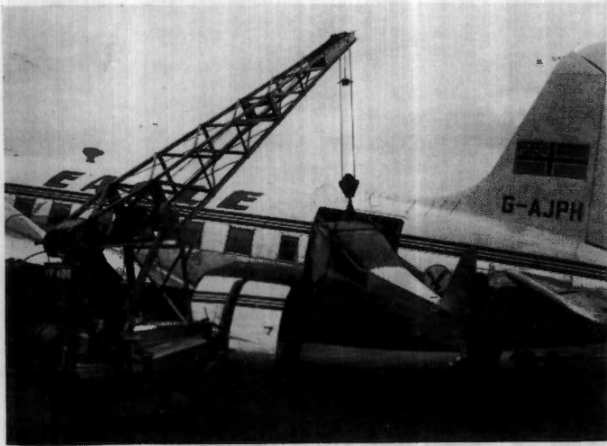
An Auster being loaded into the new Eagle Viking Freighter. Note the double freight doors, one being a quickly detachable stress panel.
